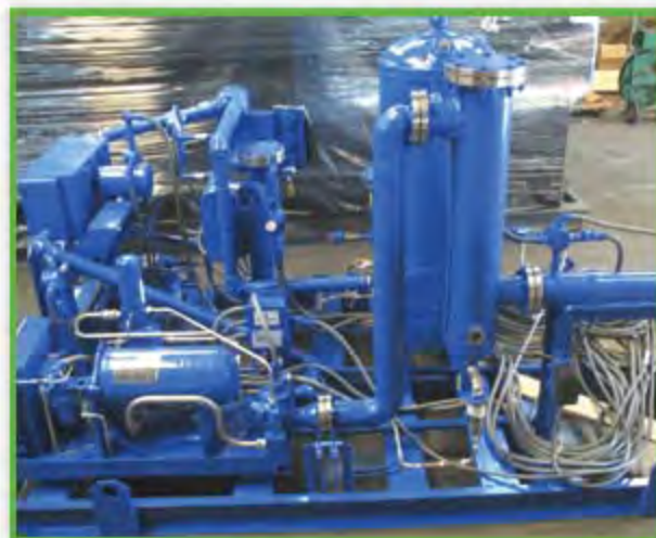
A PIONEER Model R150A-PP complete with COPELAND/EMERSON Scroll Gas Compressor with Pre & Post Gas Cleaning
